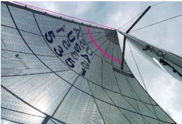
**NOT ENOUGH SAG:** In light winds on a J/24—these photos were taken in 6 to 8 knots—headstay sag is crucial for developing power in the genoa, which in turn generates pointing ability. This sail, set on a tighter headstay, has less depth, and the position of the maximum draft is further aft on the sail. A boat with a sail set this way will likely struggle to keep pace upwind in light air.
