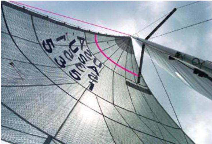
**OPTIMUM SAG:** A looser headstay helps create a more powerful genoa shape with a deeper entry, a farther forward maximum draft, and a flatter trailing edge. This creates a powerful shape that provides both maximum height and speed in underpowered conditions.
