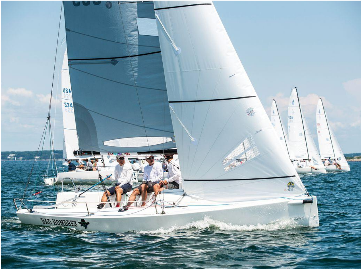
In light air, stream the telltales, set up the boat for maximum speed, and make heel-angle adjustments with crew movement. Paul Todd/ Outside Images
