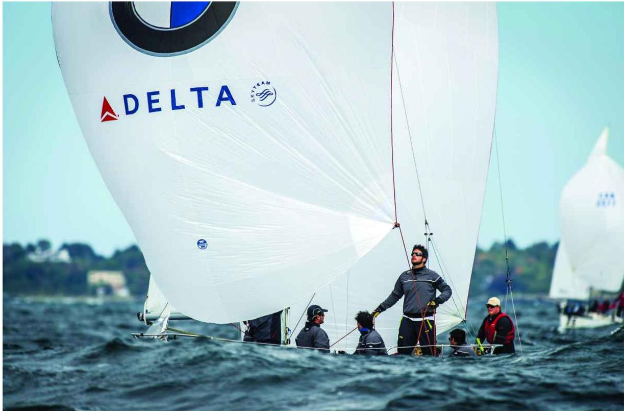
In run mode, wind flows vertically in the spinnaker, entering near the head and exiting from the foot.
