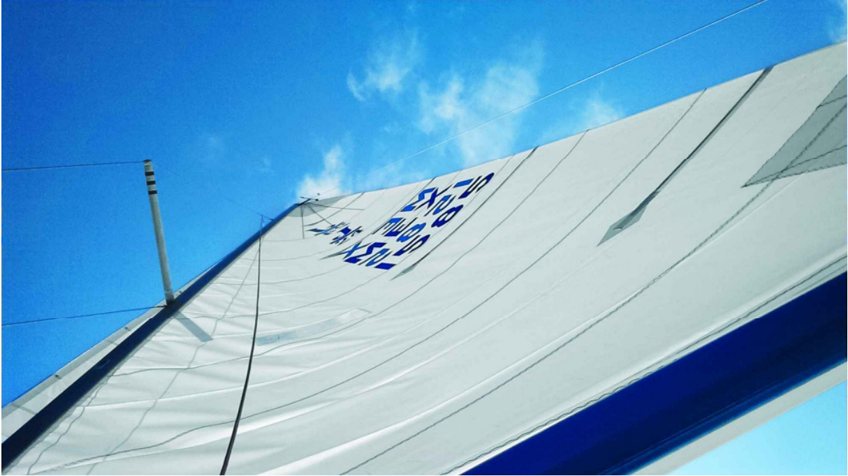
When the backstay is tensioned, the main is noticeably flatter, especially near the top-third of the sail, creating a depowered shape.
